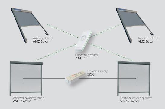
AMZ Z-Wave and VMZ Z-Wave awning blinds are connected to the ZZ60 power supply installed in the main switchboard of the building. The ZRW7 wall keypad controls AMZ Z-Wave and VMZ Z-Wave awning blinds.
