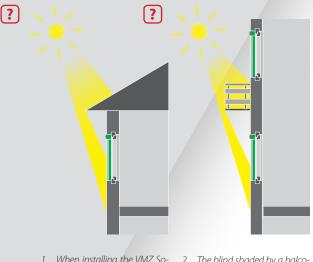
When installing the VMZ Solar, VML Solar and VMB Solar blinds under balconies or canopies it is required to purchase an additional power panel.
